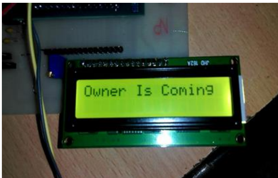
Fig 4.4 : LCD Screen display – reply of owner to system
